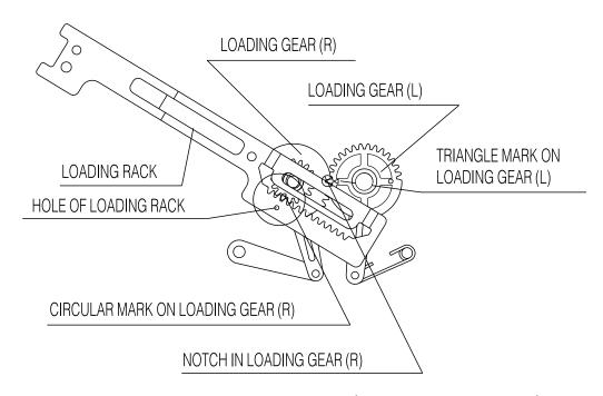
Fig.3-9 ASSEMBLY OF the R.L LOADING ASS'Y & LOADING RACK ASS'Y
